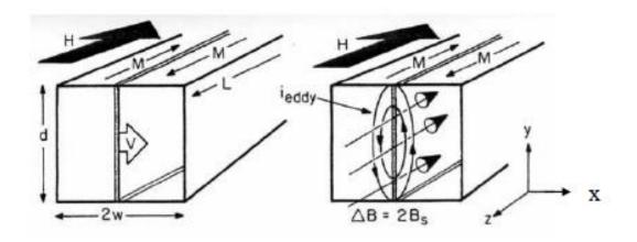
Note that the more conductive the material is, the higher its losses.
